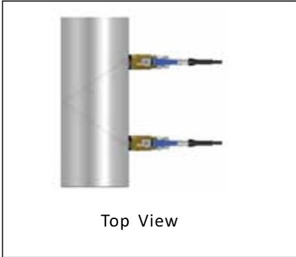
Z method measuring pipe size: 100mm-3000mm
