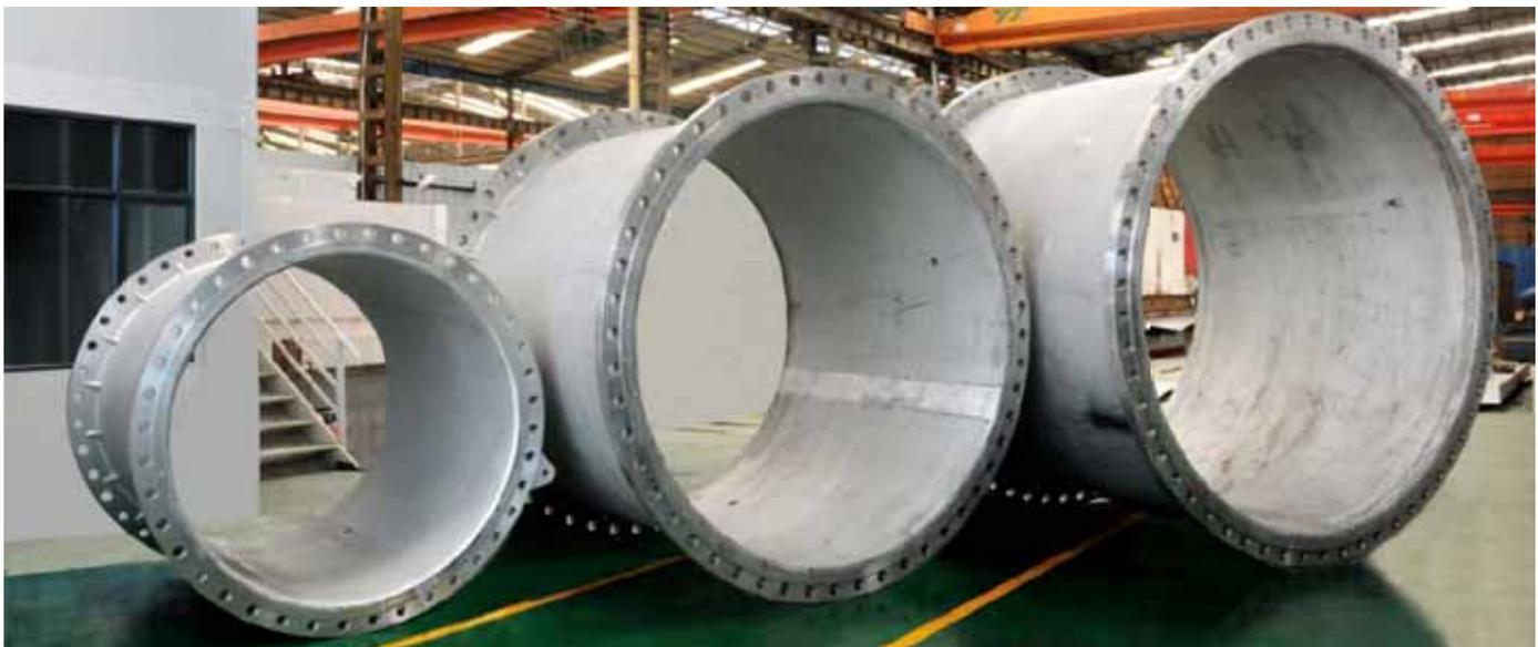
We have a 3000m<sup>2</sup> pipeline processing plant , the whole processing include the stainless steel plate cutting, reel pipe, welding and flange mating, then to polishing and pickling etc...
