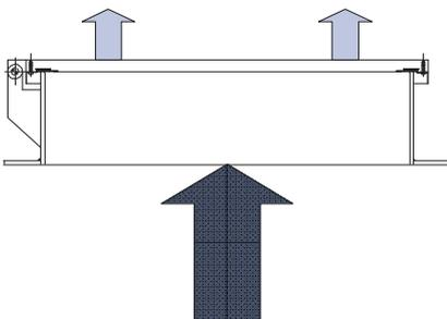
Emergency relief manways are fitted to storage tanks to allow emergency flow due to the excessive venting requirement from a fire burning around a storage tank. This eliminates a costly tank rupture, providing emergency venting from abnormal internal pressure beyond the capability of the pressure relief vent. In the event of a fire the pallet will lift at a predetermined pressure, thus supplying a large venting area.
